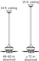
For lengths greater than 72 in., join two downrods with DR1-CP\*\* coupler
